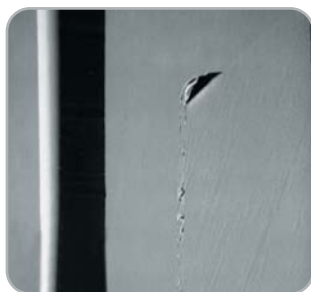
Fig. 2 SEM at 50X magnification shows intimate contact of the internal hex implant at both the beveled implant/abutment interface and the hexagonal engagement area.
