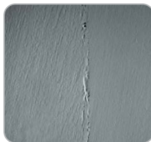
Fig. 3 SEM at 150X magnification displays the mechanical interlock in the hexagonal engagement area between the flats of the implant and abutment.
